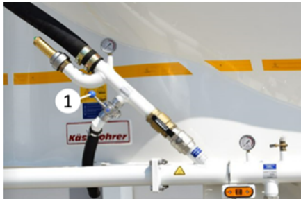
Air discharge valve
