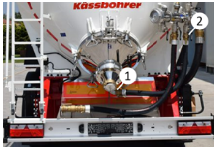
Fluidiser air line and valve
