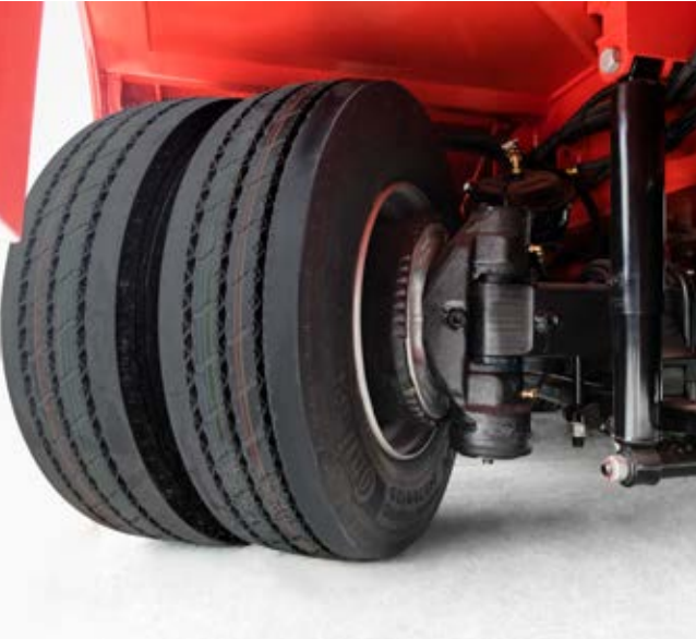
ENHANCED STEERING UP TO 42 DEGREE WITH INHOUSE DEVELOPED HYDRAULIC STEERING
