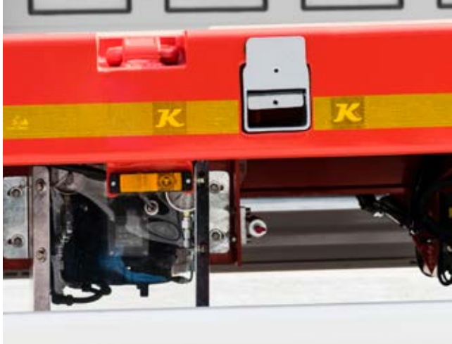
INCREASED LIFESPAN & DECREASED SERVICE COST AUTOMATIC CENTRAL LUBRICATION UNIT
