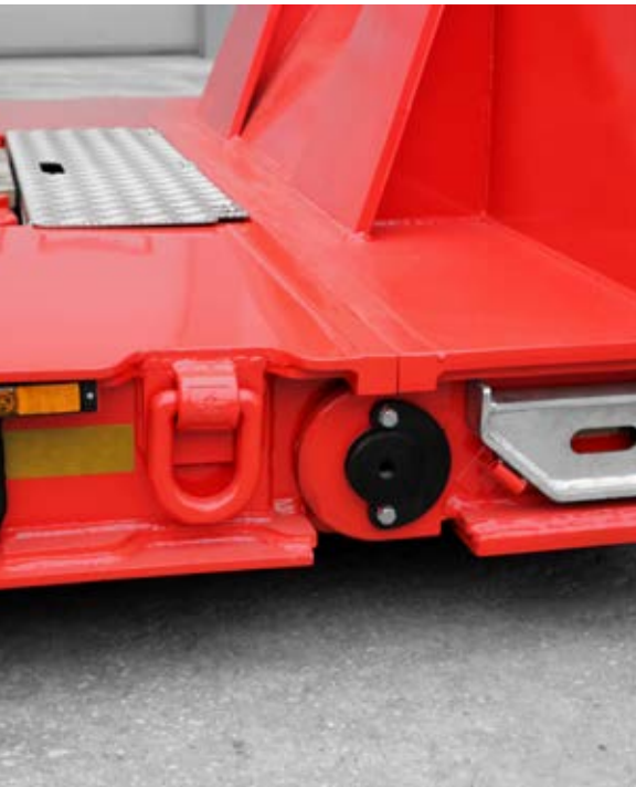
PINNED OR WELDED POOL-REAR BOOGIE CONNECTION TO BE ABLE TO HAVE DESIRED LEVEL OF IMPACT ON LOAD DISTRUBITION
