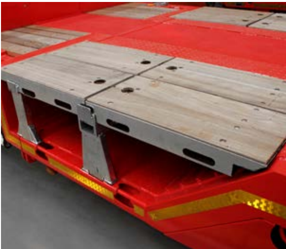
INCREASING LOAD FACTOR STEEL REINFORCED HARDWOOD DRIVE-ON WHEEL RECESS COVERS
