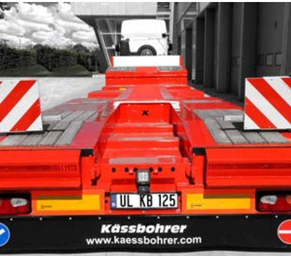
WITHIN LEGAL LIMITS FOR HIGHER LOADS, THANK TO WIDE AND DEEP EXCAVATOR ARM RECESS
