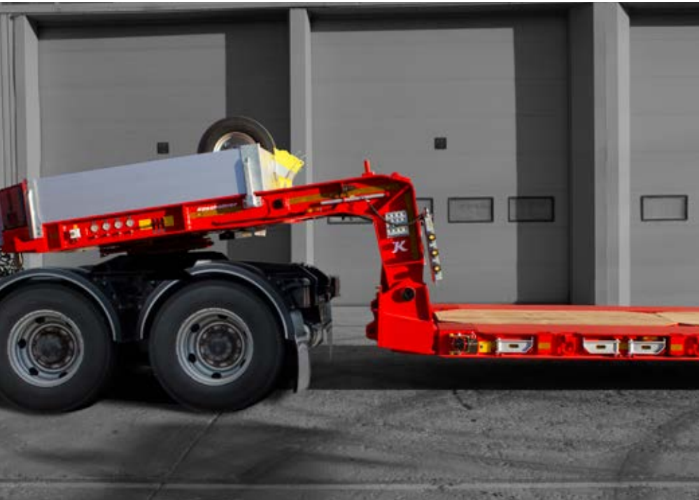
HYDRAULIC ADJUSTABLE GOOSENECK TO BETTER UTILIZE LOAD DISTRUBITION AND TO COUPLE WITH ANY TRUCK
