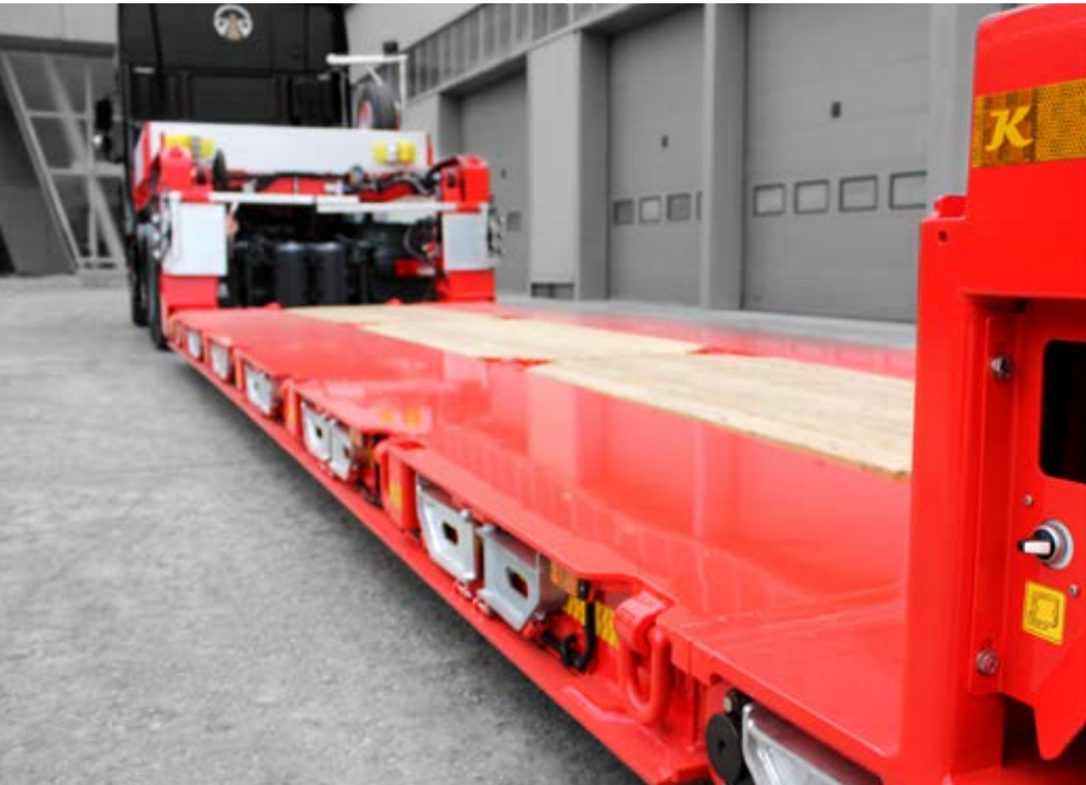
3 PIECE DETACHABLE HARDOOD FEATURING 4 UNITS OF LASHING RINGS ON EACH
