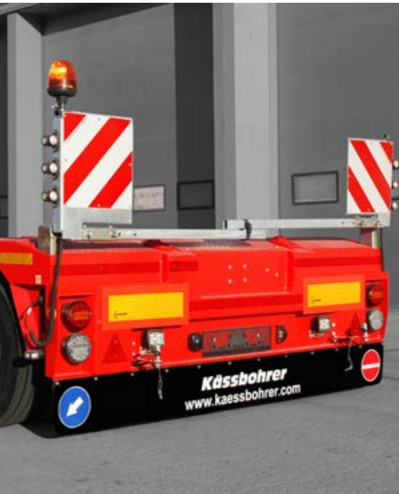
4 UNITS OF EXTENDABLE WARNING PLATES WITH LED POSITIONING LAMPS AS STANDARD
