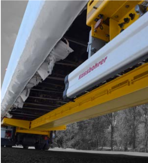
ROBUST BOX PROFILE CHASSIS CONSTRUCTION
