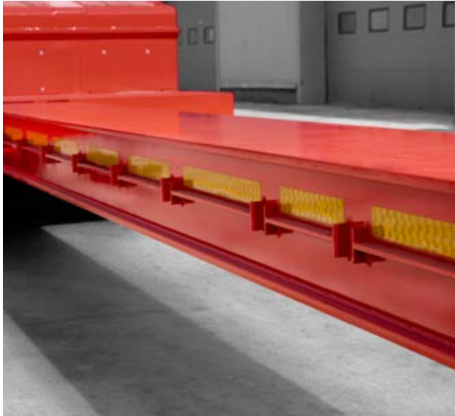
6.200 MM EXTENSION AND LOCKING POSITIONS ON EACH 500 MM
