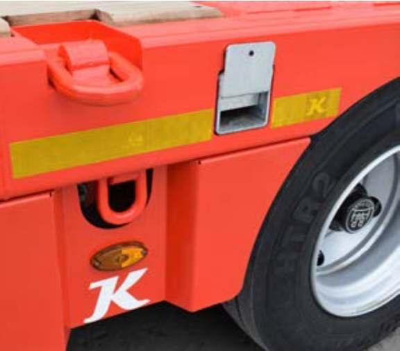
13.4 TON CAPACITY FORGED LASHING RINGS
