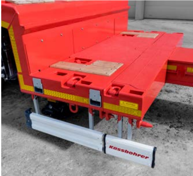
CONTAINER LOCKS, PILLAR POCKETS, LASHING RINGS AND EXTENSION BRACKETS ENSURES SAFEST LOAD TRANSPORTATION
