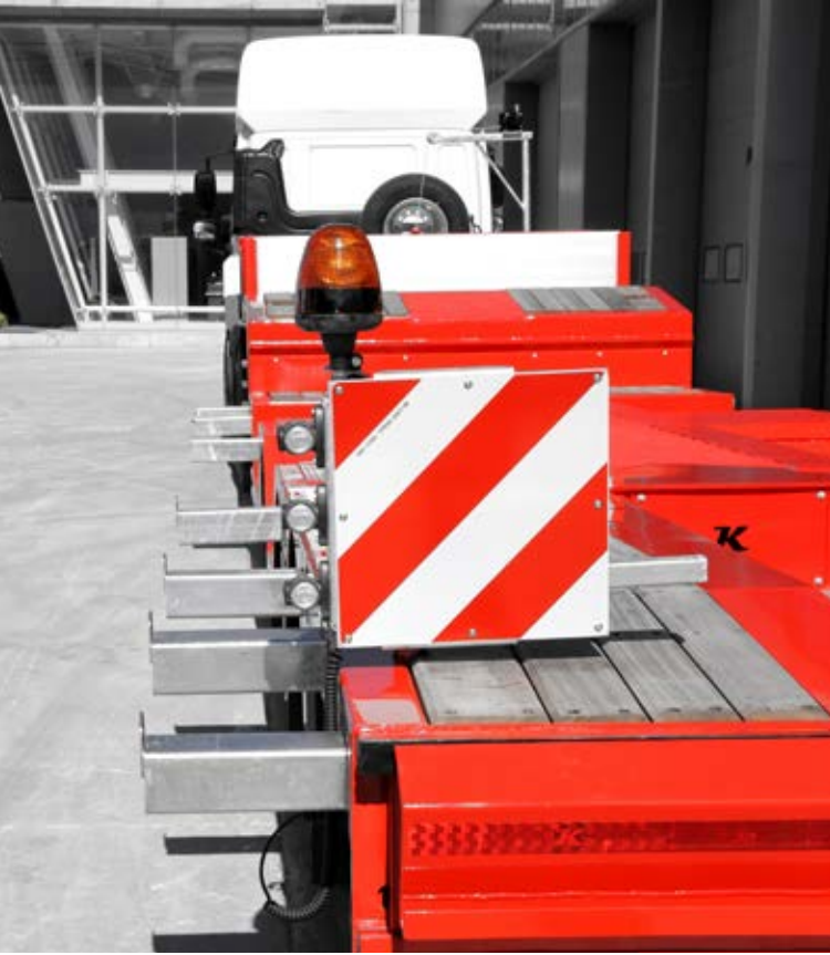
UP TO 600MM LOADING WIDTH 10x2 UNITS OF LATERAL EXTENSION
