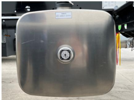
*Serbatoio diesel in alluminio*
