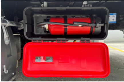
Unlocking The fire extinguisher cabinet
