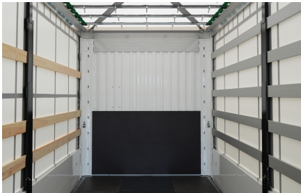
Plywood construction for protection from impacts
