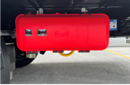
Fire extinguisher box
