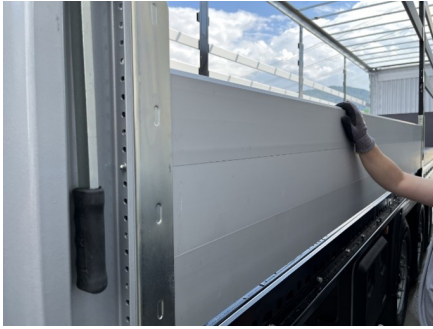
V-type aluminum side rows mounted on top of each other
