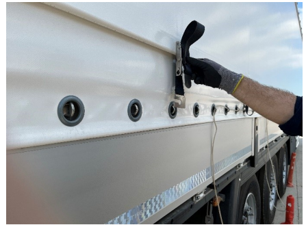
Curtain tensioner open state
