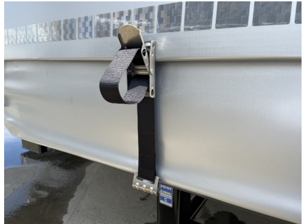
Curtain structure without board
