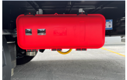
Fire extinguisher cabinet
