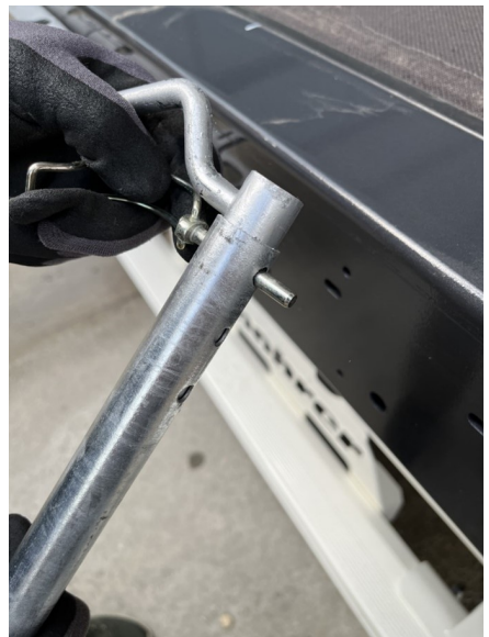
Sliding roof pull cane lock pin
