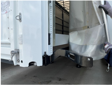
Removing the curtain pipe
