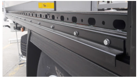
Metal forklift barrier
