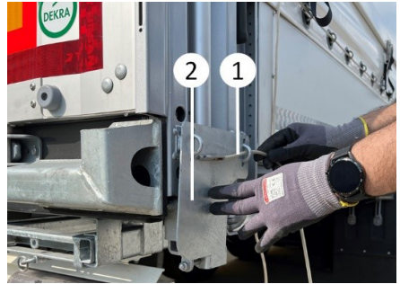
Custom cable removal
