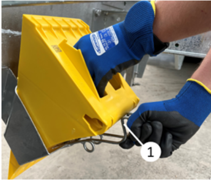
Removing the wheel chock from holders:
