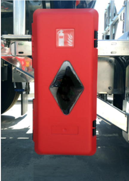
Fire Extinguisher Box
