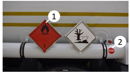
Warning plate, emergency button label
