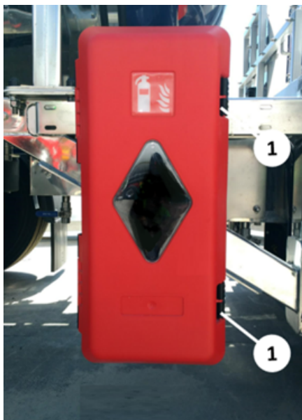
Fire extinguisher cabinet
