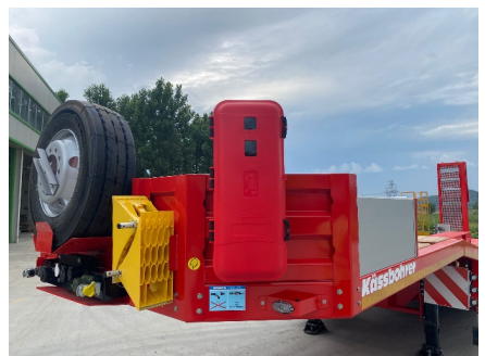
Fire Extinguisher Box
