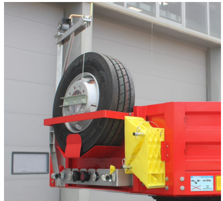
Spare tire lowering crane
