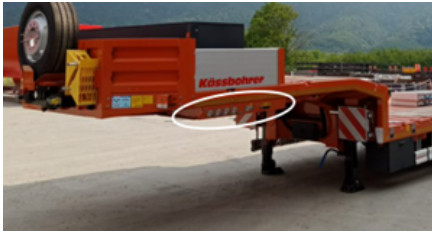
The location of the control panel
