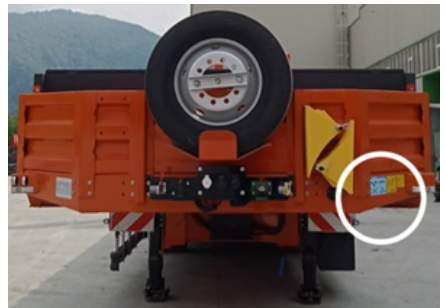
The location of battery switch
