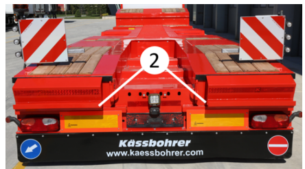
The nails that on bumper zone to place ramps
