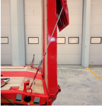
The ramp chain
