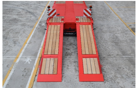
Hard wood floor ramp
