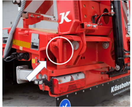
Ramp safety lock
