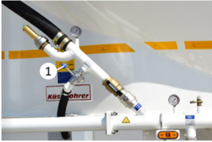
Air discharge valve
