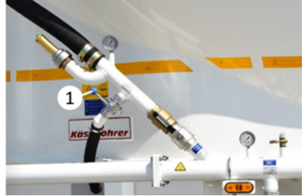
Air discharge valve
