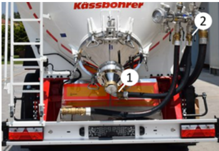
Fluidiser air line and valve
