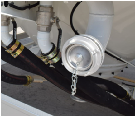
Side air line connection
