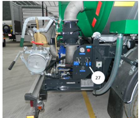
Tank ventilation valve
