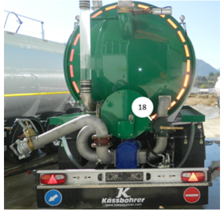
Discharge pump inlet line
