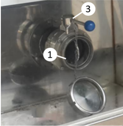
Discharge port, butterfly valve
