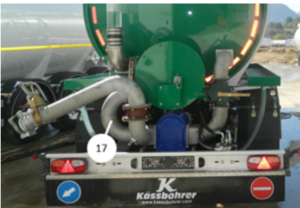
Tank mixing pump inlet line
