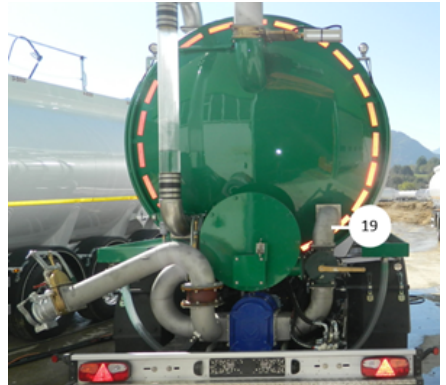
Tank mixing pump outlet line
