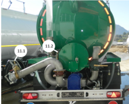
Manual control gate valve
