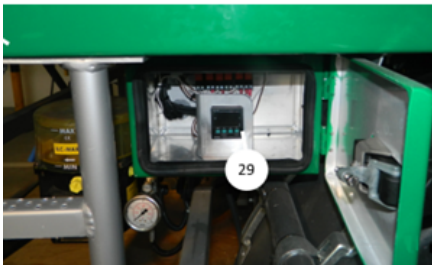
Central lubrication electronic counter system
