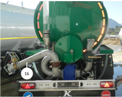
Discharge pump outlet line
