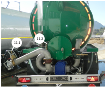
Manual control gate valve
