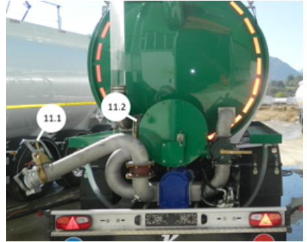
Manual control gate valve
