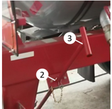
Gate valve extension lever
