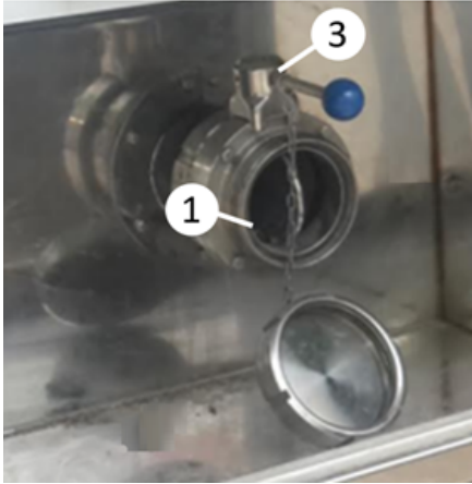
Discharge port, butterfly valve
