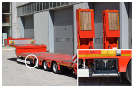
The location of the control cabinet on the lowbed vehicle
