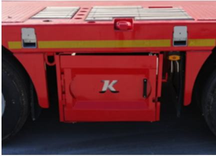
Ramp storage cabinet
