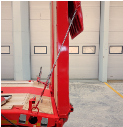
The ramp chain
