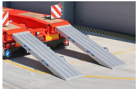
The aluminum ramps that usable on bumper zone
