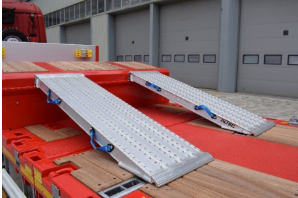
The aluminium ramps that usable on gooseneck
