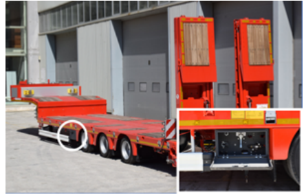
The location of command cabinet
