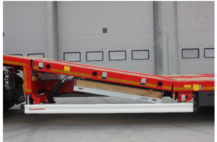
The upper position of ramp
