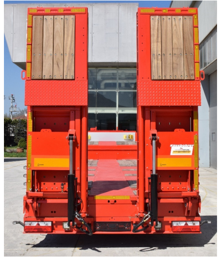
Hard wood floor ramp
