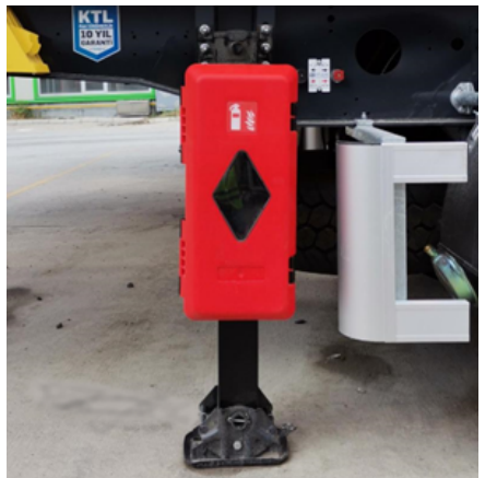
Fire extinguisher box
