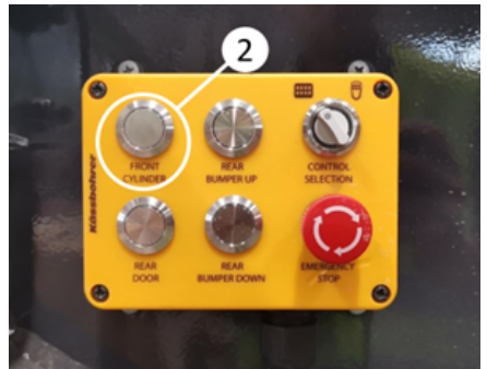
Lifting the tub with pushing front cylinder button on the remote control device
