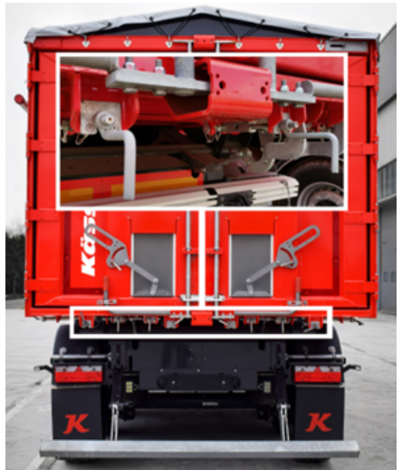
Location of tightening locks
