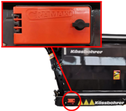
Tarpaulin control unit location
