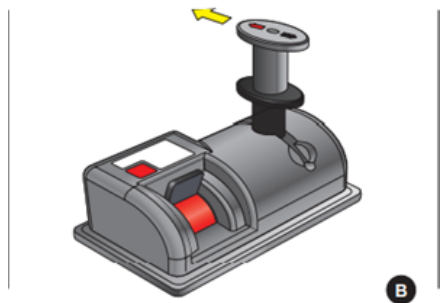
pushing the joystick in the direction of the red arrow at the top
