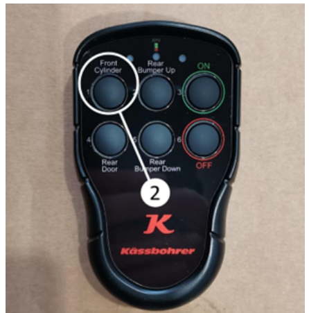
Lifting the tub with pushing front cylinder button on the remote control device
