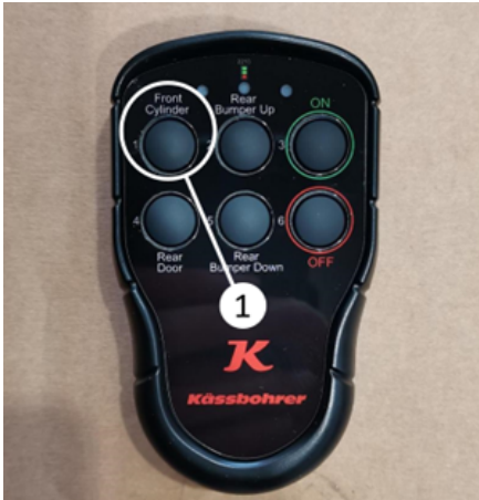
Lowering the tub with pushing front cylinder button on the remote control device
