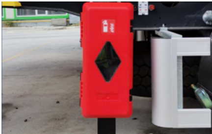
Fire extinguisher cabinet
