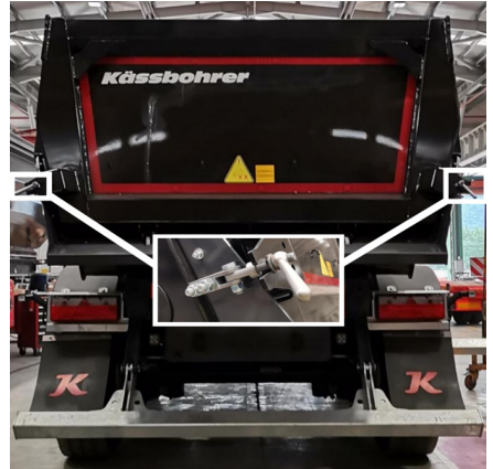
Location of tightening locks
