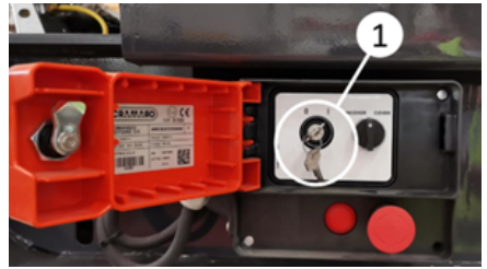
Turning the control unit on
