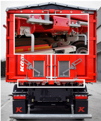
Location of tightening locks
