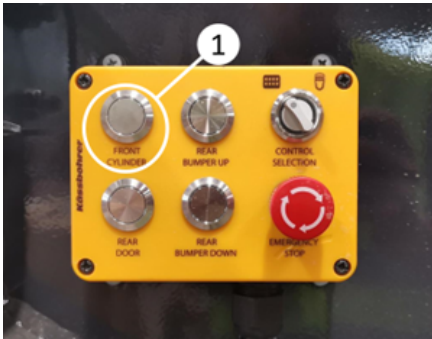
Lowering the tub with pushing front cylinder button on the remote control device
