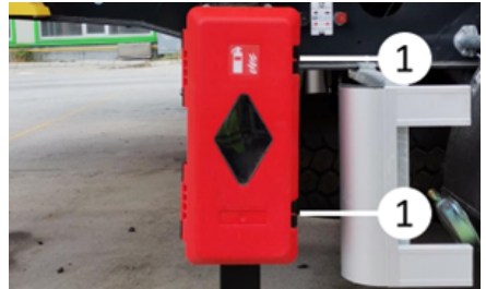
Unlocking The fire extinguisher cabinet
