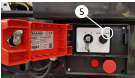
Closing the tarpaulin with the control unit
