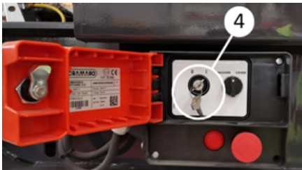
Turning the control unit on
