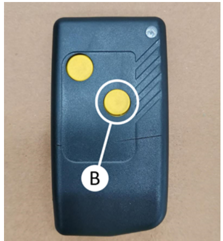
Opening the tarpaulin with the remote control device
