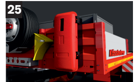
25 Fire Extinguisher Box
