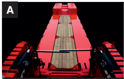
A Double or Central Box Beam
